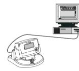
Run the application software. The vellow LED on the cradle blinks to indicate that the communication is active. Do not remove the logger while the LED is blinking.
