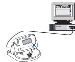
Run the application software. The yellow LED on the cradle blinks to indicate that the communication is active. **Do not remove the logger while the LED is blinking**.
