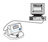
Run the application software. The yellow LED on the cradle blinks to indicate that the communication is active. **Do not remove the logger while the LED is blinking**.
