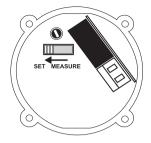
• With a small screwdriver adjust the setpoint trimmer to display the desired value in the 0 to 50°C or -20 to 20°C range (based on the model).
