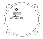
• With a small screwdriver adjust the setpoint trimmer to display the desired value in the 0 to 50 °C or in the 32 to 122°F range for the **Celsius or Fahrenheit** models, respectively.
