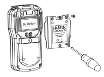
Unscrew the three screws on the rear of the meter, remove the battery compartment cover and replace the 9V battery with a new one, while observing the correct polarity. Make sure the battery contacts are tight and secure before replacing the cover.
